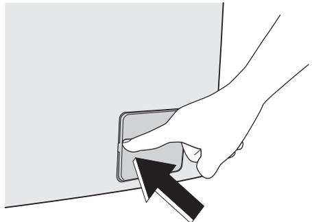
**Warning!** When the appliance is in use and depending on the programme selected there can be hot water in the pump. Never remove the pump cover during a wash cycle, always wait until the appliance has finished the cycle, and is empty. When refitting the pump cover, ensure it is securely re-tightened so as to stop leaks and young children being able to remove it.
